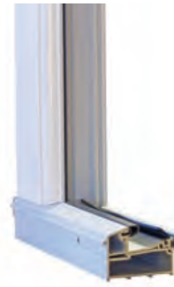
Stormguard Plus Rebated Threshold Distance from bottom of door leaf to bottom of threshold - 20mm. Available in Silver only. (Not wheelchair accessible)
